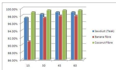
Fig. 1. The graph represents the adsorption rates of sawdust, banana fibre and coconut fibre at every 15 min intervals
