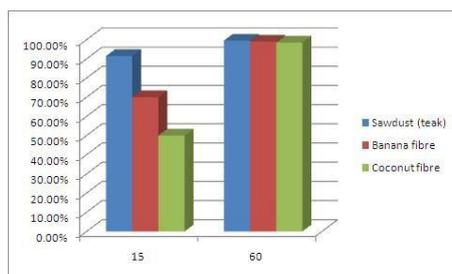
Fig. 2. The graph represents the adsorption rates of dye by sawdust, banana fibre and coconut fibre at 15 and 60 min
